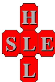
The rough edges between the components in the SHEL diagram are symbolic of the fact that the **mismatch** between an individual and these components is important. These possible mismatches warrant special attention by the marine investigator because mismatches in the system may point out safety deficiencies. Examples of mismatches between a person and other components include:
