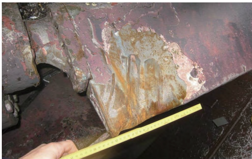
Figure 16.1 damage sustained on the starboard stabiliser fin SOURCE DNV, Investigation report(AIBN)
