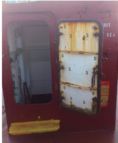
Figure 4.2 The weather-tight door on the fore-castle deck 출처 Investigation report(HKSAR)
