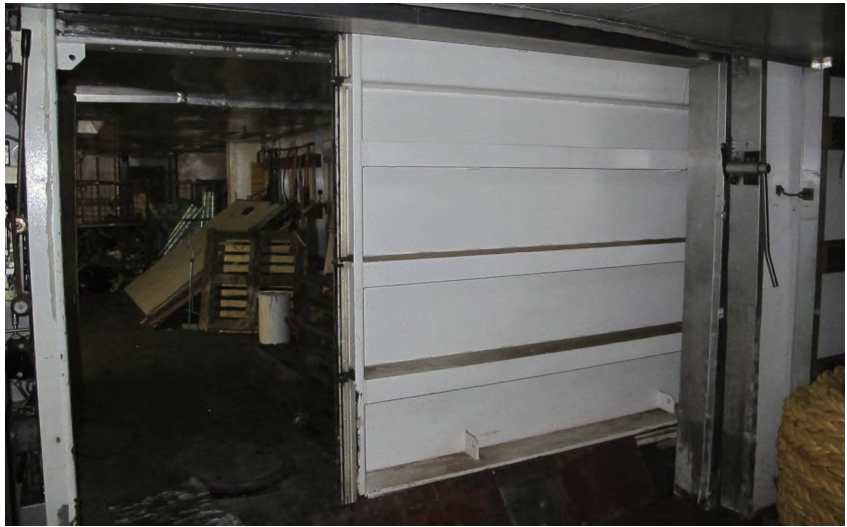
Figure 16.2 The watertight sliding door between cargo hold no 1 and cargo hold no 2 출처 Investigation report(AIBN)
