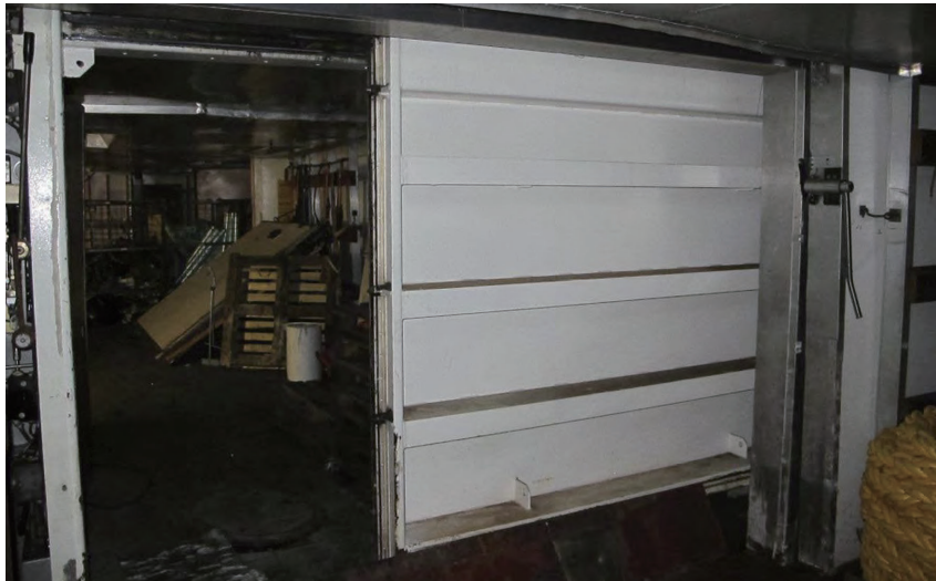
Figure 16.2 The watertight sliding door between cargo hold no 1 and cargo hold no.2 SOURCE Investigation report(AIBN)
