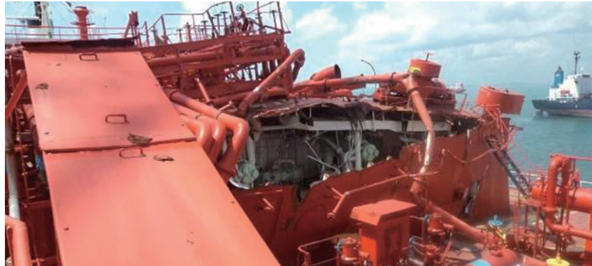
Figure 9.1 Photo of the accident(Fwd cargo compressor Room) SOURCE Investigation report(Panama Maritime Authority)
