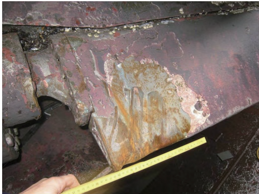
Figure 16.1 damage sustained on the starboard stabiliser fin 출처 DNV, Investigation report(AIBN)
