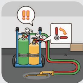
Shut off the oxygen valve after using the welding cutter
