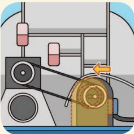
Adjust the pulley position to loosen when replacing the V-belt
