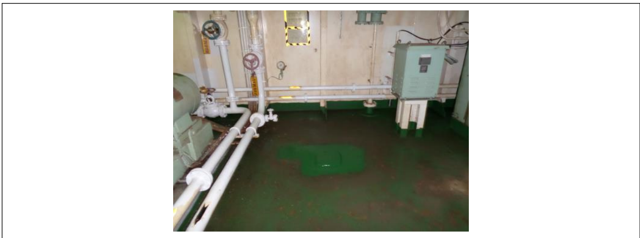
[Figure 17] Doubling the floor plate of the deck store on the bow (3Q2015 Hull Inspection Report)
