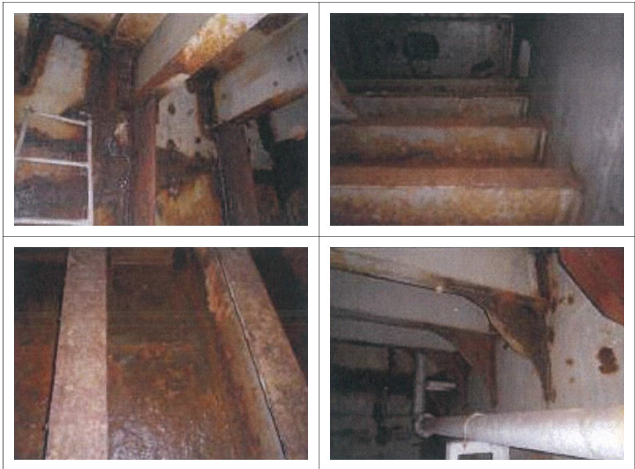
[Figure 15] VTs (c) under cargo holds (4Q2013 Hull Inspection Report)
