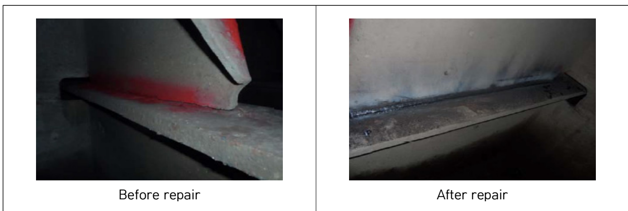
[Figure 18] Cracked trans. web frame of WBT No. 4 (P) (3Q2015 Hull Inspection Report)
