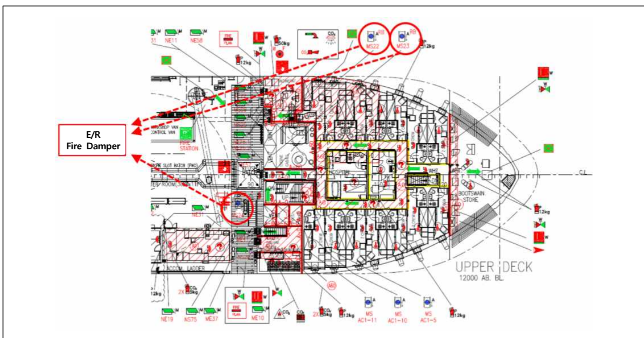
<Figure 4> Location of fire dampers in Responder (Upper deck)
